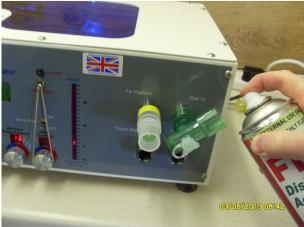
Set Merlin to Run so that the ventilator cycles continuously. Spray a 2-second burst of F10 into the open green connector on the return stroke of the piston. This is when the piston is filling with gas and sucking air from the Gas-In port. Do this at least 6 times. This will allow F10 aerosol to be pulled directly into Merlin and leave a small pool of F10 in the green connector.
